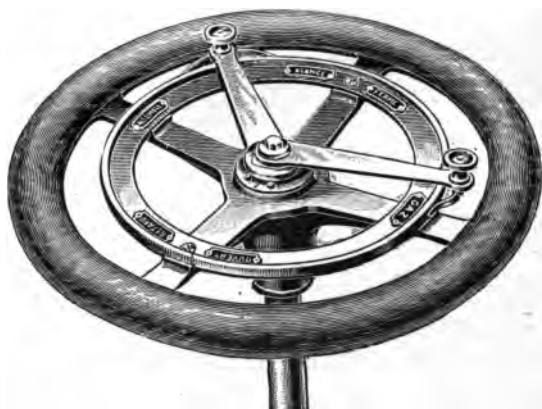
FIG. 232—Steering Wheel and Control Levers of the Vinot Motor Carriage. The throttle and spark levers work on opposite arcs of the ring. Both turn clockwise for high speed adjustments, and counter clockwise for low speeds, as indicated.
